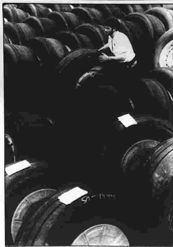
ONE MORE GO-AROUND — A worker selects one of the huge commercial aircraft tires which will be retreaded at Air Treads Inc.'s Atlanta, Ga., plant. A subsidiary of Goodyear, Air Treads can retread tires this size up to six times.
